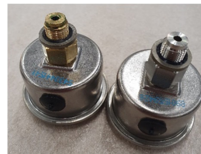
Old gauge with brass connector to the left, and new with stainless steel connector to the right.
